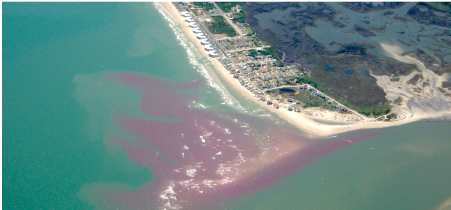
Aerial picture of the ebb delta region in New River inlet. The picture shows the Rhodamine WT distribution during the release done the 8th of May during the RIVET experiment. Image courtesy of Prof. Falk Feddersen and Prof. Robert Guza from SOI.
