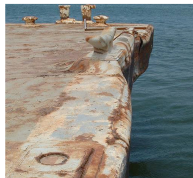
(a) (b) Figure 3. Full-scale barge impact tests at St. George Island (2004): a) overview of tests; b) deformed bow following testing
