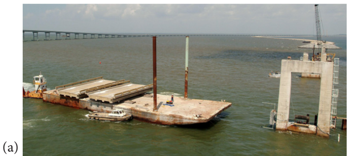
(a) (b) Figure 3. Full-scale barge impact tests at St. George Island (2004): a) overview of tests; b) deformed bow following testing
